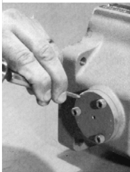
MARKING TRUNNION LOCATION
