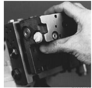
Fig. 50-102 - Install Control Housing
