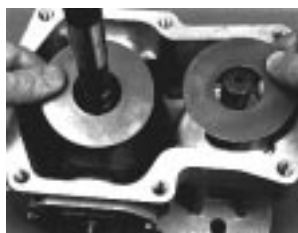
Fig. 65-29 - Install Thrust Plates
