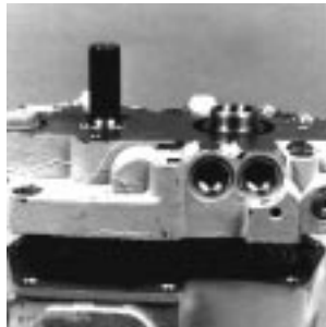
Fig. 65-2 - Remove Center Section and Valve Plates
