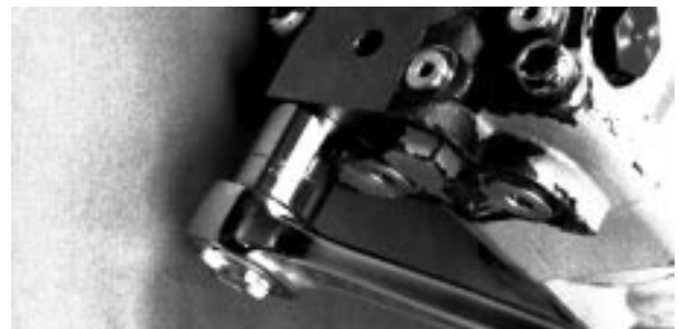
Fig. 50-31 - Remove Charge Relief Valve Plug (U)
