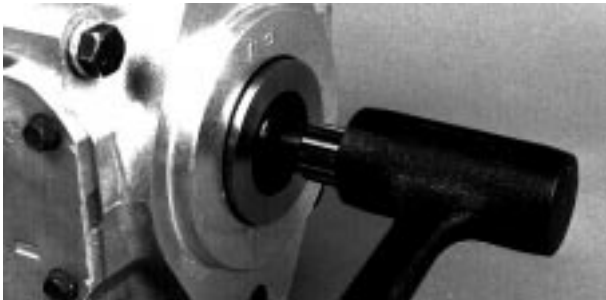
Fig. 50-3 - Tapping Shaft with Soft Hammer to Remove Seal Carrier from Housing (PV / PT / MF)
