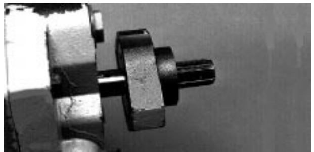
Fig. 50-23 - Installing Charge Pump Cover with Shaft Seal (U)
