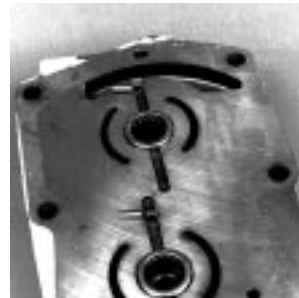
Fig. 65-32 - Install Valve Plate Pins
