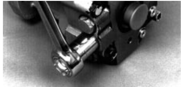
Fig. 50-37 - Remove Filter Bypass Reverse Flow Check Valve Plug (U)
