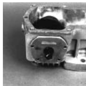
Fig. 65-21 - Install Trunnion Seal Cover
