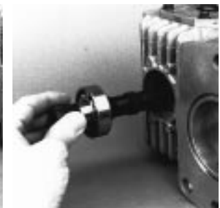
Fig. 65-14 - Remove Pump Shaft and Bearing
