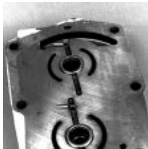
Fig. 65-5 - Remove Valve Plate Pins
