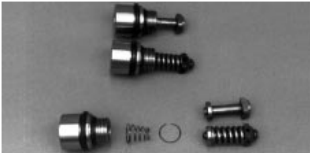
Fig. 50-12 - Check and Relief Valve Components (PV / PT)
