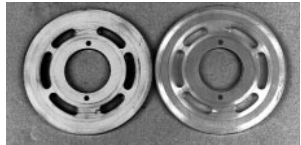
Fig. 61-30 - Pump Valve Plates
