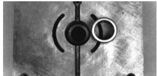
Fig. 62-6 - Drive Coupling in place in Center Section for Installation of Second Needle Bearing (Tandem Pump)
