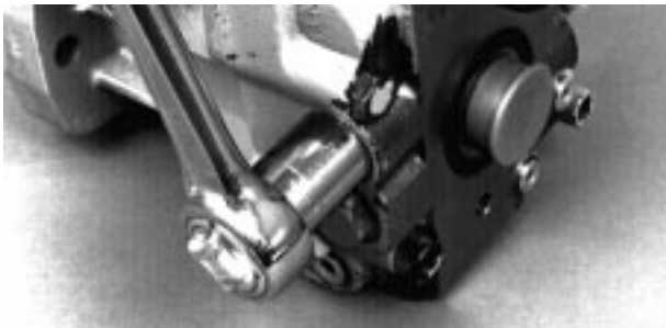
Fig. 50-35 - Remove Filter Bypass Valve Plug (U)
