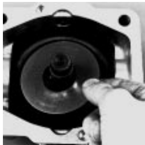
Fig. 61-25 - Install Thrust Plate
