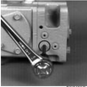
Fig. 50-10 - Remove Check and Relief Valve Plug (PV)
