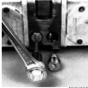
Fig. 50-11 - Remove Check and Relief Valve Plug (PT)
