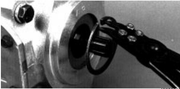
Fig. 50-2 - Remove Seal Carrier Retaining Ring (PV / PT / MF)
