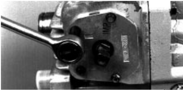
Fig. 50-24 - Remove Trunnion Seal Cover (U)
