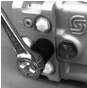
Fig. 50-13 - Remove Charge Relief Valve Plug (PV)
