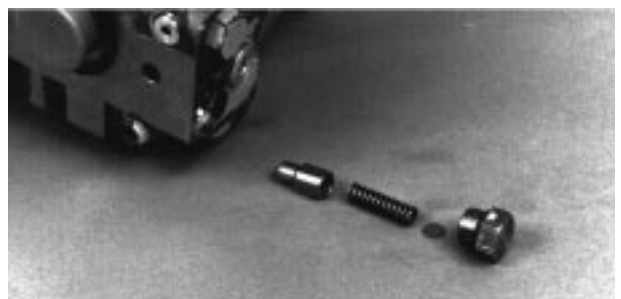
Fig. 30-8 - Charge Relief Valve (U)
