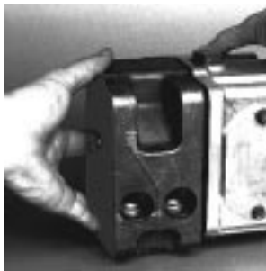
Fig. 62-11 - Assemble Rear Pump Section to Center Section
