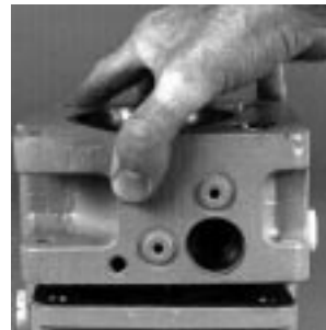
Fig. 61-31 - Install End Cap Gasket and End Cap
