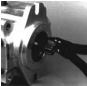
Fig. 61-24 - Install Shaft Seal Cover
