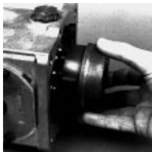
Fig. 61-27 - Install Cylinder Block Kit
