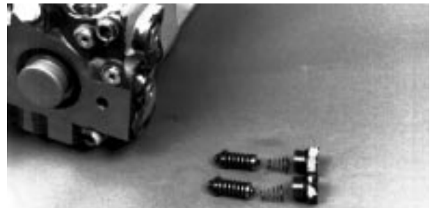
Fig. 50-30 - Check / High Pressure Relief Valves (U)
