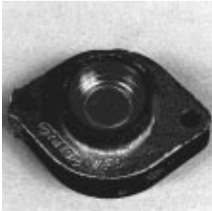
Fig. 50-42 - Bearing Installed in Charge Pump Cover (U)
