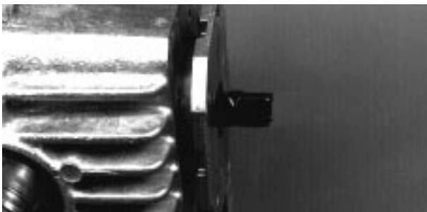
Fig. 50-26 - Install Trunnion Seal Cover (U)
