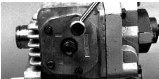
Fig. 50-27 - Torque Trunnion Seal Cover Screws (U)
