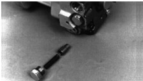
Fig. 30-11 - Filter Bypass Valve (U)
