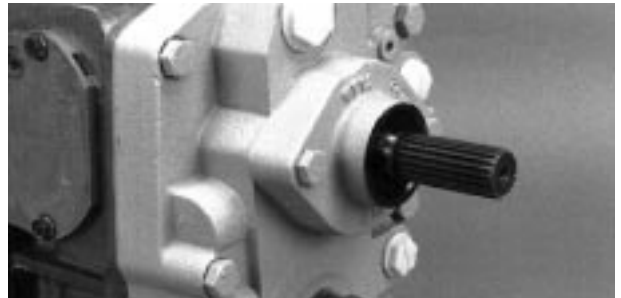
Fig. 50-22 - Shaft Seal Installed (U)
