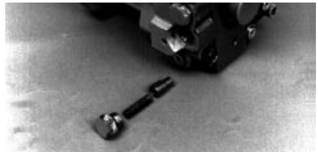
Fig. 50-38- Filter Bypass Reverse Flow Check Valve (U)
