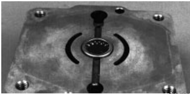
Fig. 61-14 - Needle Bearing Installed in End Cap
