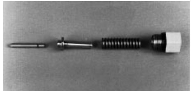
Fig. 50-18 - Easy-Ride Valve Components (PV)
