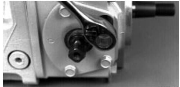
Fig. 50-6 - Remove Trunnion Seal Cover (PV / PT)
