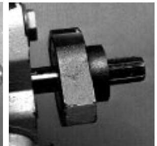
Fig. 50-40 - Remove Charge Pump Assembly (U)
