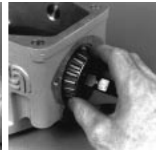
Fig. 61-18 - Install Trunnion Bearings (Tapered Roller)
