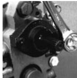
Fig. 50-39 - Remove Charge Pump Cover Screws (U)
