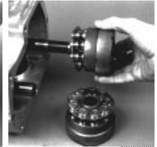
Fig. 65-31 - Install Cylinder Block Kits
