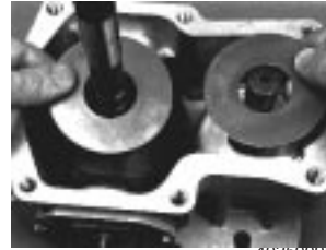
Fig. 65-8 - Remove Thrust Plates
