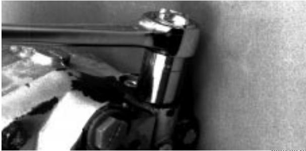
Fig. 50-33 - Remove Heat Exchanger Bypass Valve Plug (U)
