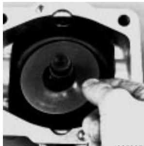
Fig. 61-7 - Remove Thrust Plate
