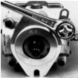
Fig. 61-2 - Remove Housing Screws
