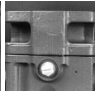
Fig. 61-32 - End Cap Installed
