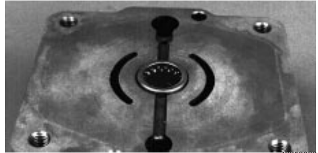
Fig. 62-5 - Needle Bearing Installed in Center Section (Tandem Pump)
