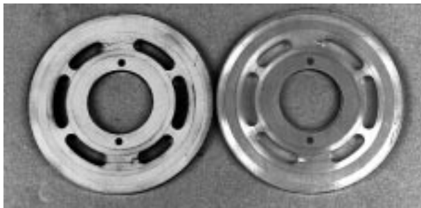
Fig. 62-9 - Pump Valve Plates
