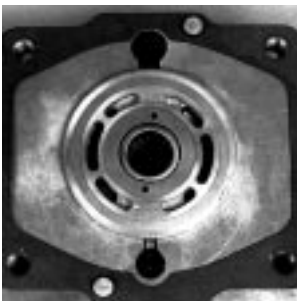
Fig. 62-10 - Install Center Section Gasket
