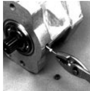
Fig. 65-10 - Remove Bearing Retaining Pin
