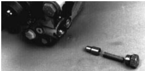
Fig. 30-10 - Heat Exchanger Bypass Valve (U)
