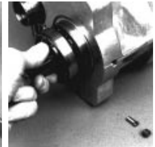
Fig. 65-11 - Remove Motor Shaft Assembly
