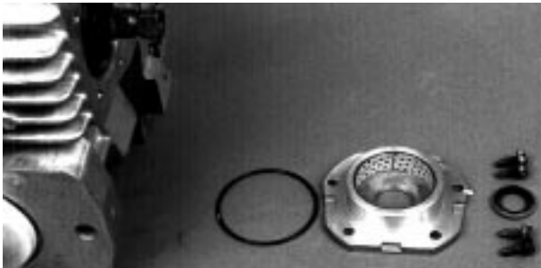
Fig. 50-25 - Trunnion Cover Components - Journal Bearings (U)
