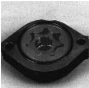
Fig. 50-44 - Install Gerotor Assembly in Pump Cover (U)
