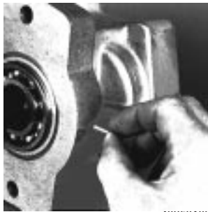
Fig. 65-27 - Install Bearing Retaining Pin
