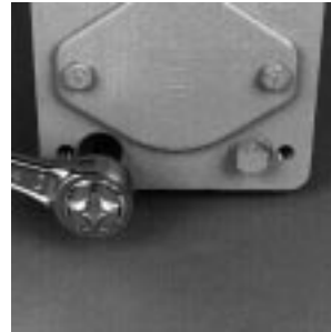
Fig. 50-16 - Remove Easy Ride Valves (PV)
