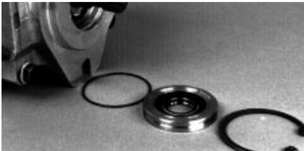
Fig. 50-4 - Shaft Seal Removed (PV / PT / MF)
