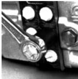
Fig. 50-14 - Remove Charge Relief Valve Plug (PT)
