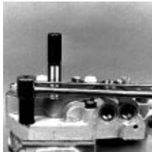
Fig. 65-38 - Torque Center Section Screws
