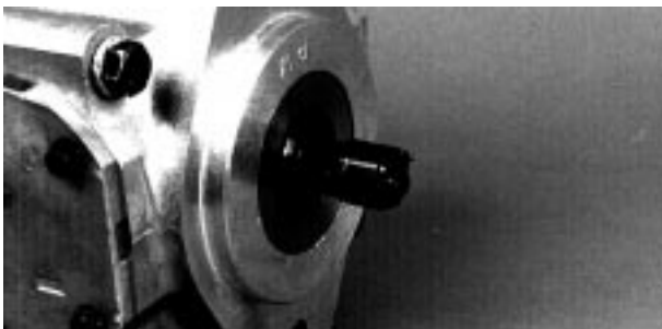
Fig. 50-5 - Install Seal Carrier with O-Ring (PV / PT / MF)
