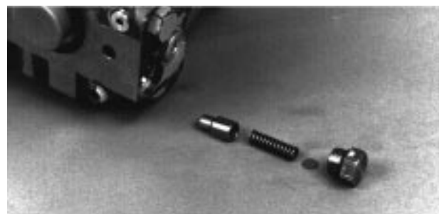
Fig. 50-32 - Charge Relief Valve Components (U)
