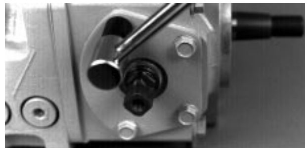
Fig. 50-9 - Torque Trunnion Seal Cover Screws (PV / PT)
