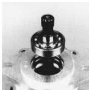
Fig. 61-9 - Remove Shaft and Bearing
