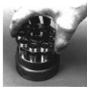
Fig. 65-30 - Install Piston Assemblies into Cylinder Block
