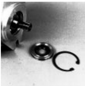
Fig. 61-8 - Remove Shaft Seal Cover
