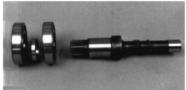
Fig. 65-12 - Components of Motor Shaft Assembly
