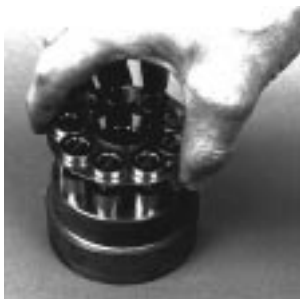
Fig. 61-26 - Install Piston Assemblies into Cylinder Block
