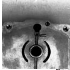
Fig. 61-28 - Install Valve Plate Pin
