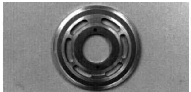
Fig. 65-35 - Motor Valve Plate
