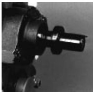
Fig. 50-49 - Installing Shaft Seal (U)
