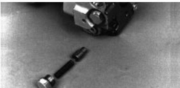
Fig. 50-36 - Filter Bypass Valve (U)
