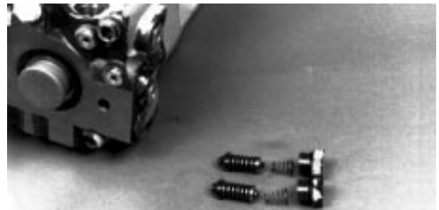
Fig. 30-6 - Check / High Pressure Relief Valves (U)
