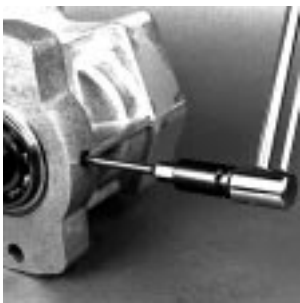
Fig. 65-28 - Install Pipe Plug
