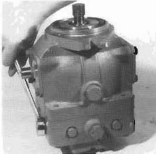
Fig. 29 - Remove Check and Relief Valve Plug (PV)
