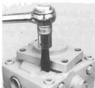
Fig. 27 - Remove Charge Check Valves
