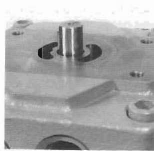
Fig. 39 - Install New Drive Key
